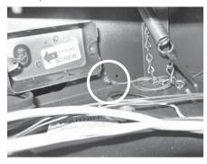
25) Connect one end of the supplied green ground wire to the lug with the nut and washer from the kit.
