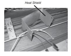
**28)** Plug the DC spark generator wires to the DC Sparker.
