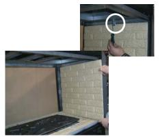
Remove the burner by removing the 4 screws.
