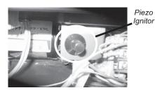
Remove the Piezo Ignitor by unscrewing the nut at the back of the mounting bracket.
