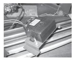
**29)** Connect the ground wire to the DC Sparker mounting bracket.
