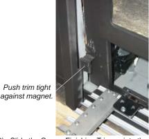
Slide the Corner Finishing Trim up into the slot in the top flange of the fireplace. Push tight against the magnet at the base of the unit.
