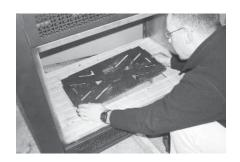
8) Remove the Side Base Brick Panels and finally the Long Base Brick Panels.
