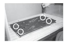
Slide the burner assembly away from the orifice and lift out.
