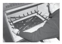
Remove the side brick clip in the top of the firebox and then slide the Side Brick Panel out. The brick panels are very fragile - handle with care.
