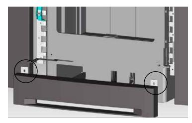
4) Lift fan housing up off pins on floor of unit.
