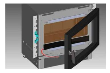
**NOTE:** For Masonry installation make sure that the firebox is level with the hearth using non-combustible materials and no more than 1/2 to 1 inch of the levelling bolt.
