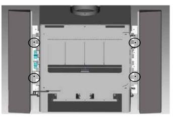
7) Loosen the two (2) top screws (with 3/16" allen key) on the left and right brackets on the unit as shown below.
