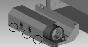
7) Slide back the protect sheath on the wiring - disconnect the black, red and white wires.
