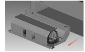
6) Remove 3 screws to remove fan heat shield.
