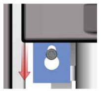
10) Tighten both screws once all three cast pieces are level.
