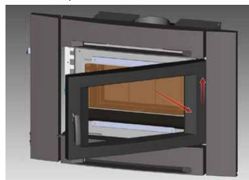
Remove two (2) screws (with 3/16" Allen Key) to remove lower cast sur-3) round - set aside on a soft surface.
