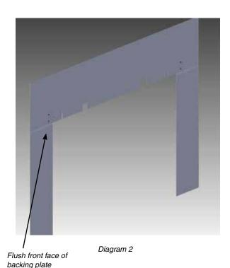
3) Install 2 clips to the back of the top cast faceplate with hex bolts. If the unit is already installed - remove the top cast faceplate from the unit if access is too difficult - see 'Cast Faceplate Installation' in the owners manual for instructions.
