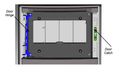
6) Remove the glass from the door and flip it around 180° - so the painted strip is at the bottom of the door.
