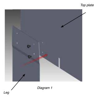
2) The pointed end of the screws should be facing the front of the backing plate.
