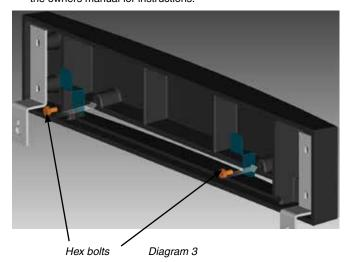
4) Slide the backing plate over the clips on the back of the cast top. There are notches in the backing plate where it sits on the clips. If the stove is installed - slide it out at least 6" to install the backing plate.
