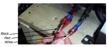
8) Disconnect the ground wire located on the left side of the fan housing.
