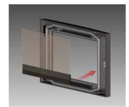
7) Flip the handle around 180° and reattach to the door with 2 botls.
