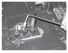
Remove burner orifice with a 1/2" wrench, while using a 9/16" wrench to hold onto the elbow behind the orifice and discard orifice.
