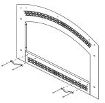
4) Place the emblem over the emblem design on the surround. Insert the studs through the holes. To secure them first put on the split lock washer and then the nut and tighten.
