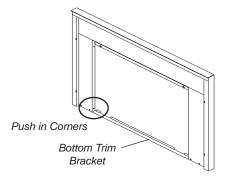
Completely secure faceplate to the unit by securing 4 screws to the Left and Right Side Trim.
