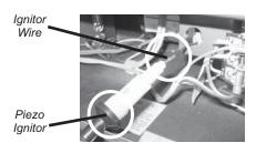
29) Disconnect the ignitor wire from the Piezo Ignitor and connect it to the D.C. Sparker.
