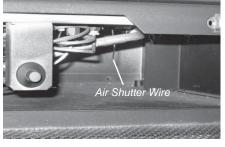
Straighten adjustment wire.
