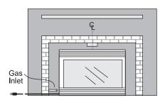
3) Locate the center point where the vent will pass through the chimney above the appliance. Move the appliance into the exact location where it is to be installed. Ensure that the Insert is level.
