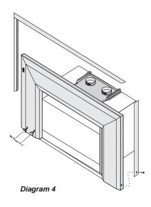
10) Attach the faceplate panels to the insert body using the 4 remaining black screws. Refer to Diagram 5.
