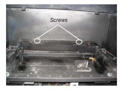
**10)** Remove the 12 screws holding the Access Panel in place.
