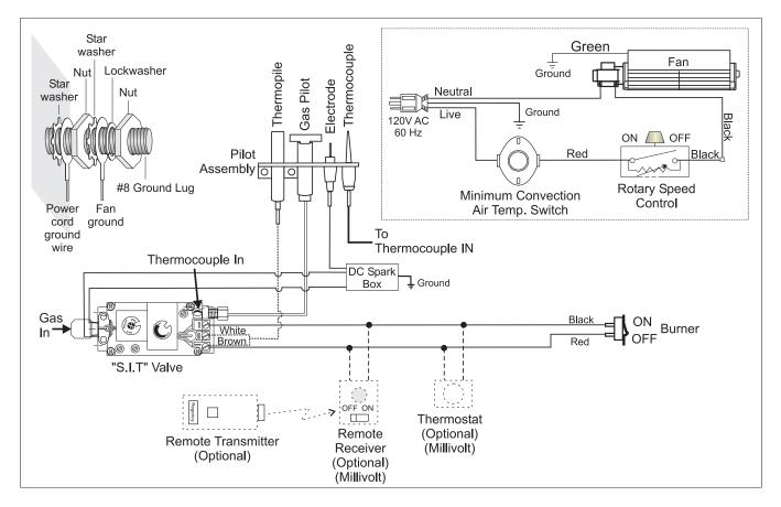
\*For installation of the DC Spark Box refer to the LP Conversion instructions in this manual.
