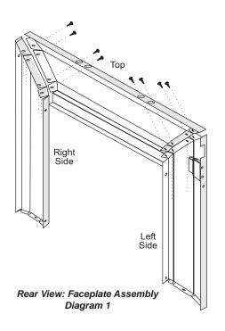
Using the connectors provided, join the left side trim (with the ON/OFF switch) to the top trim. Diagram 2. Connect the right side trim to the top trim.
