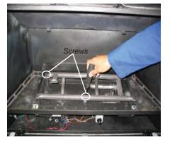
9) Remove the rear log support by unscrewing the 2 screws.
