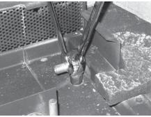
Burner Orifice Removal
