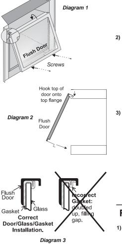
Secure door by fastening with two screws located at bottom of glass frame (refer to Diagram 1).
