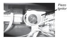
**28)** Remove the Piezo Ignitor by unscrewing the nut at the back of the mounting bracket.
