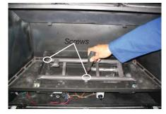
10) Remove the rear log support by unscrewing the 2 screws.
