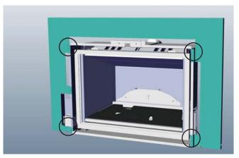
Diagram 4–Backing Plate Removal Units L390E/HZI390E/L540E/ HZI540E
