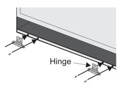
6) Place Bottom Frame near hinge. Flip hinge over Bottom Frame and secure with 3 screws each.
