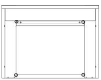
Install the Top Frame by hooking it onto the two screws at the top of the full screen door. It is held in place by magnets.
