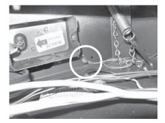
**32)** Connect one end of the supplied green ground wire to the lug with the nut and washer from the kit.
