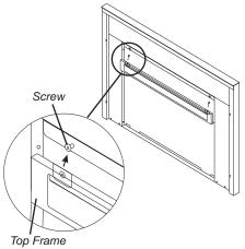
Install Spring Hinges to the Left and Right Side of the bottom of the firebox using 2 screws per hinge.
