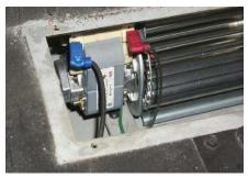
Remove the 2 screws from the fan bracket.
