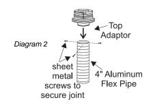
4) Pass the flex pipe down through the center of the chimney system, and center the adaptor on the top of the chimney pipe. Drill four 1/8" diameter holes through the adaptor and into the chimney top. Insure that you are in fact, drilling into the metal on the chimney. Twist-lock the Termination Cap onto the Adaptor. (Diagram 3 and 4).
