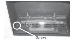
4) Unscrew the pilot orifice with the Allen key and replace with the LPG pilot orifice in the kit and replace pilot cap.
