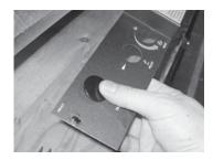
Attach the DC sparker generator connector to the valve with a screw.
