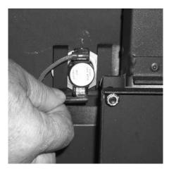
10) Feed the short red and black wires through the small hole at the base of the unit.
