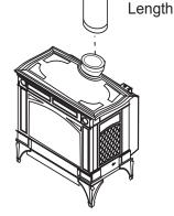
When using Rigid Vent other than Simpson Dura-Vent, 3 screws must be used to secure rigid pipe to adaptor.
