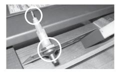
3) Plug up the Piezo hole with the plastic bushing.
