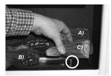
The Front Right Log front edges should be placed parallel against the front edge of the burner.
