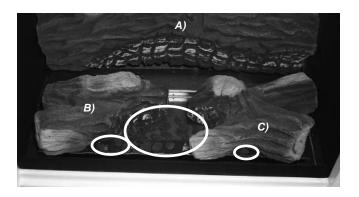
8) Test fire to ensure proper light off (make sure flame flows smoothly from one end of burner to the other). If there is any flame hesitation, check that area for any blockage of the burner ports.
