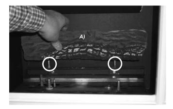
5) Place the 2 front logs on the front log locating pins. Ensure the back of both logs rest against the tabs.
