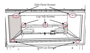
7. Remove burner by removing 2 screws in locations shown below.
