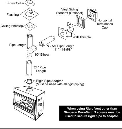
The Regency AstroCap<sup>™</sup> and Regency Riser Vent terminal are certified for installations using Regency venting systems as well as Simpson Dura-Vent® Direct Vent , American Metal Products Ameri Vent Direct Vent, Security Secure Vent®, Selkirk Direct-Temp. AstroCap<sup>™</sup> is a proprietary trademark of Regency Fireplace Products. Dura-Vent® and Direct Vent are registered and/or proprietary trademarks of Simpson Dura-Vent Co. Inc.
