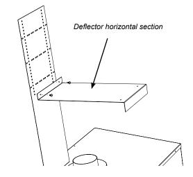
4. If the deflector extender is required, install with 2 screws, extend to desired length before tightening screws.
