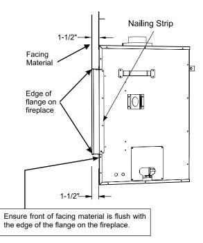
5) If material such as brick, stone, etc extends past the faceplate depth 1-1/2", when finishing around the faceplate, the minimum opening dimensions noted below must be adhered to ensuring for the removal of the faceplate and for the safe operation of this appliance.
