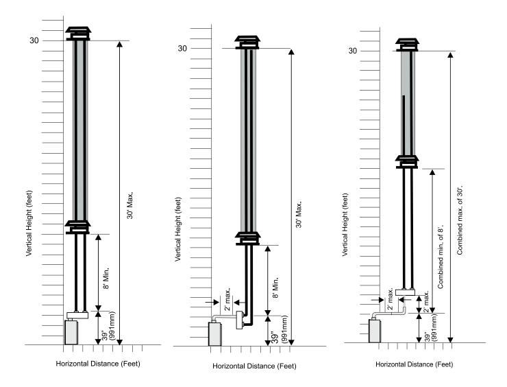
The shaded area in the diagrams show the allowable vertical terminations. Restrictor Position Set 0-3" Factory Setting
