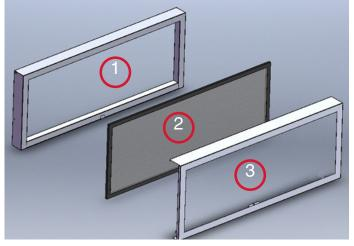
2. Remove screws from inner side of the inner door trim and discard screws and the brackets. (Brackets not shown). Remove the screen mesh from inner door trim.
