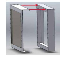
5. Bend the center tab up and secure with a screw to attach the inner door frame/safety screen assembly to the inner door trim
