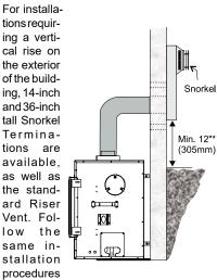
as used for standard Horizontal Termination. NEVER install the snorkel upside down.
