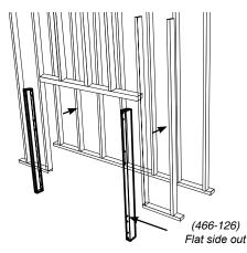
5. Secure horizontal steel header stud (466-128) with 2 screws per side as per diagram.
