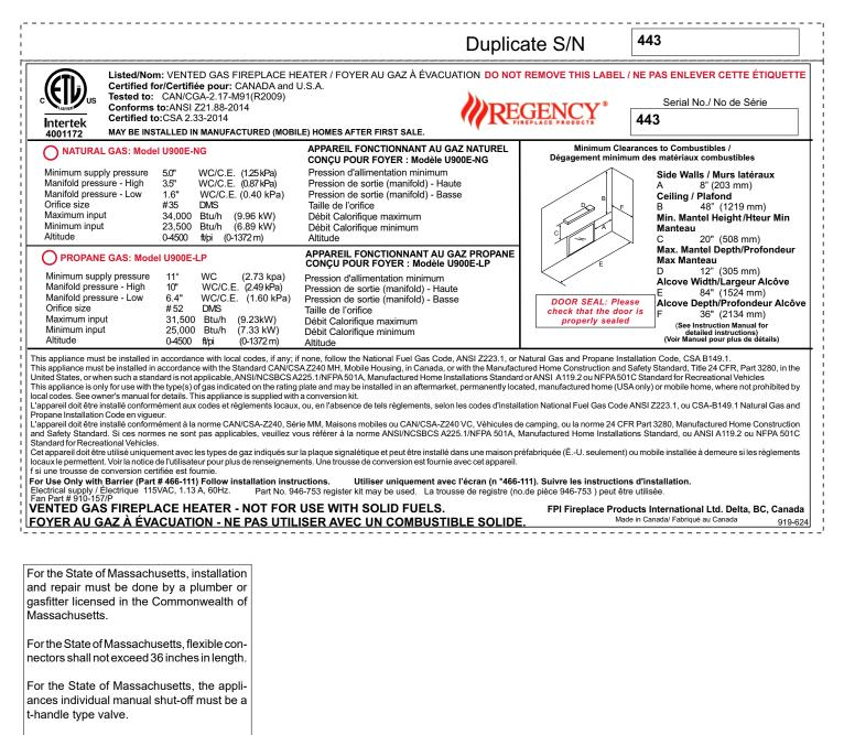
The State of Massachusetts requires the installation of a carbon monoxide alarm in accordance with NFPA 720 and a CO alarm with battery back up in the same room where the gas appliance is installed.
