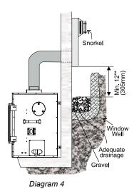
The arrow on the vent cap should be pointing up. Insure that the 1-1/2" clearances to combustible materials are maintained (Diagram 4). Install the termination cap.
