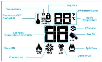
Figure 2: Transmitter LCD Display
