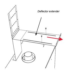
5. If there is any excess material on the horizontal section of the deflector, it can be folded down at the fold lines.
