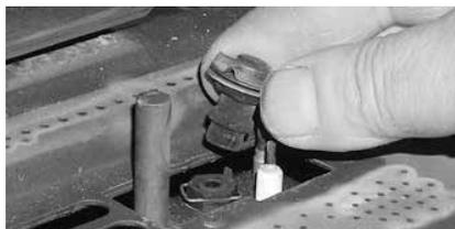
7. Unscrew the pilot orifice with the allen key; then replace the LP pilot orifice and reinstall the pilot cap provided in the kit
