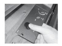
4) Attach the DC sparker generator connector to the valve with a screw.
