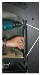
Door Bracket attaches with 2 screws.
