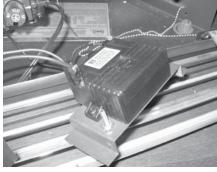
**10)** Connect the ground wire to the DC Sparker mounting bracket.
