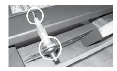
Plug up the Piezo hole with the plastic bushing.
