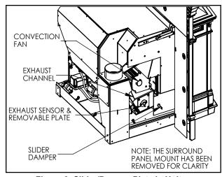
Figure 6: Slider/Damper Plate in Unit.
