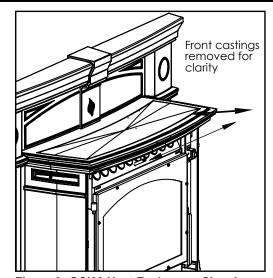
Figure 9: GCI60 Heat Exchanger Cleaning.
