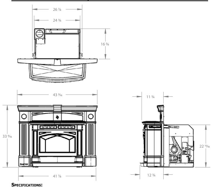
Input rating when using: Wood Pellets/Corn - 55,000BTU (16.1KW•hr) & Wheat/Barley - 53,000BTU (15.5KW•hr). Table 1: GCI60 Specifications.
