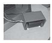
**18)** We recommend mounting the DC Sparker box onto the pedestal back cover.
