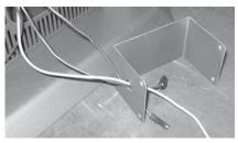
**13)** Apply the plastic bushing to the heat shield hole.
