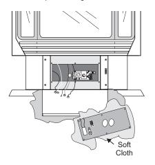
4) Remove the two outside frame pieces by removing two screws per side. See diagram below.
