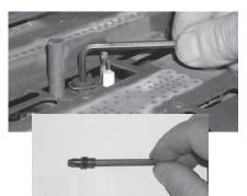
18) Remove burner orifice with a 1/2" wrench while using a 9/16" wrench to hold onto the elbow behind the orifice, then discard the orifice.
