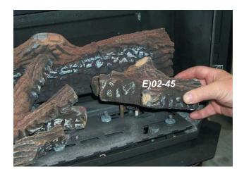
9) Place the lava rock in the area between the left and right logs, leaving a space in the middle for log (F) 02-47.
