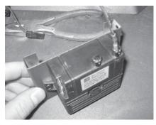
**12)** The ground wire and DC Sparker ignition go through the hole on the heat shield.
