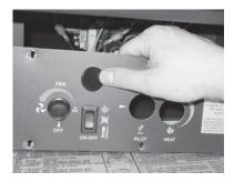
Connect the DC spark generator wires to the SIT Valve with the screw, which is provided in the kit.
