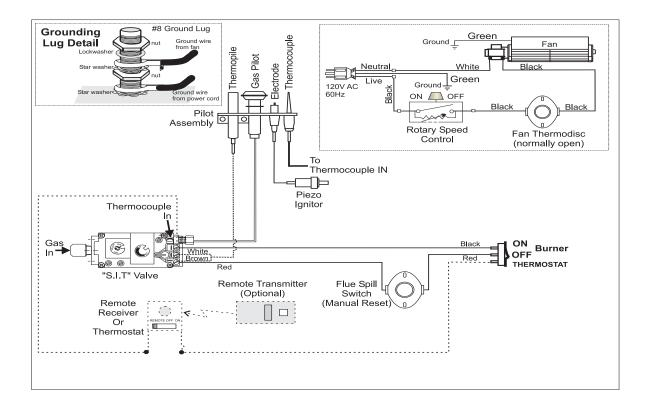
WARNING: Electrical Grounding Instructions This appliance is equipped with a three pronged (grounding) plug for your protection against shock hazard and should be plugged directly into a properly grounded three-prong receptacle. Do not cut or remove the grounding prong from this plug.
