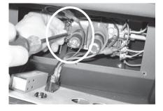
Reversing step 2 and secure the control panel back onto the stove pedestal with the screws.
