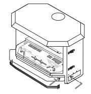
To adjust the aeration: use the allen key to turn the turning gear which will adjust the air shutter. Open the air shutter for a blue flame or close it for a yellower flame.
