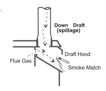
Note: If the flue is blocked or has a strong reverse flow, the thermally actuated safety switch mounted in the draft hood will automatically shut off the gas supply within about 10 minutes. If the heater turns off because of this during the spillage test, check for the cause of the lack of draft.
