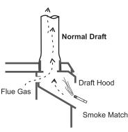
The smoke should be drawn into the draft hood. If the smoke is not drawn into the draft hood, turn the unit off and check for the cause of lack of draft.
