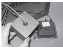
14) Connect the DC Sparker Ignition Wire to the DC Sparker.
