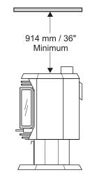
If further reduced clearances are needed, obtain requirements for construction of a protected wall from your local building authorities and their allowable reductions of the listed clearances.
