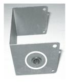
8) Run the other end of the ground wire and DC spark generator wires through the bushing on the heat shield.
