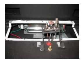
11) Remove the 2 screws that hold the fan in place and slide the fan towards the front of the unit.
