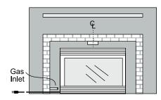
Locate the center point where the vent will pass through the chimney above the appliance. Move the appliance into the exact location where it is to be installed. Ensure that the Insert is level.
