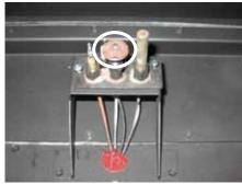
10) Unscrew the pilot orifice with the supplied allen key and replace it with the LP pilot orifice and re-install the pilot cap.
