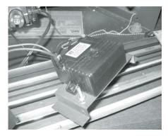
Connect the ground wire to the DC Sparker mounting bracket.
