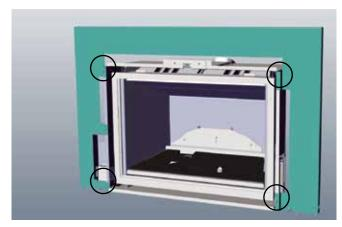
Diagram 4–Backing Plate Removal Units L390E/HZI390E/L540E/ HZI540E
