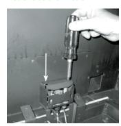
Remove the base cover by lifting up from the back and maneover out.
