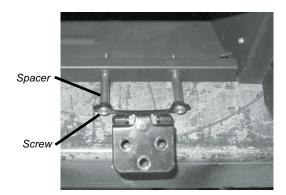
8) Align the left and right side hinge with the screw holes in the bottom louver and secure in place using 3 screws per side.
