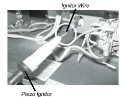
Disconnect the ignitor wire from the Piezo Ignitor and connect it to the DC Sparker.
