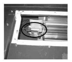
13) Lift up the left side of the fan and disconnect the ground wire shown.
