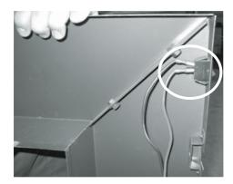
Connect the grey coated female ends of the black & red fan wires from the unit to the male ends of the fan rheostat on the left side of the faceplate as shown.
