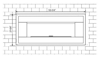
6) For material such as brick, stone, etc that extends less than 1-1/2", the minimum opening dimensions noted below must be adhered, when finishing around the faceplate. This is to ensure the removal of the faceplate and for the safe operation of this appliance.
