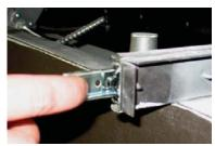
4) Push done on the black lever on the outside of the inner slide - this will release the inner slide. Pull inner slide completely out - from outer slide.
