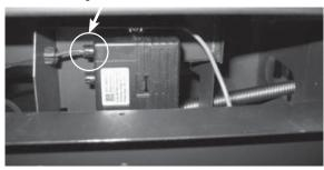
11) Remove the valve tray by undoing the 14 outer screws.
