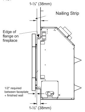
5) If material such as brick, stone, etc extends past the faceplate depth (1-1/2"), when finishing around the faceplate, the minimum opening dimensions noted below must be adhered to ensuring for the removal of the faceplate and for the safe operation of this appliance.
