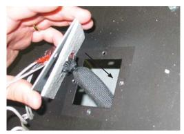
11) Remove the 2 cover plates and gaskets located in the lower front of the firebox by removing 4 screws from each plate - see below. Discard cover plates and gaskets - keep the screws.
