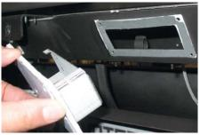
**16)** Secure the light diffuser in place with the 4 screws set aside from the cover plates.
