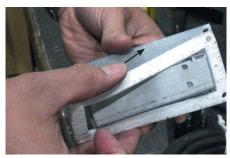
15) From outside the firebox -Install light assembly box and gasket into opening created from the removal of the cover plates open end up - as shown below.
