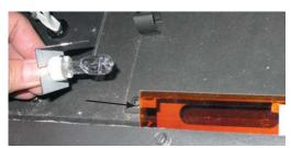
20) Secure socket to light diffuser with one screw - as shown below.
