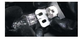
19) Install socket and bulb into light diffuser as shown below.
