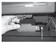
DC Spark Box mounting plate partially removed.
