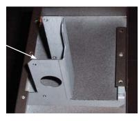
HZ42ST - install slider with flat side facing inwards -secure with 2 screws in locations shown.
