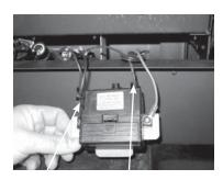
Generator Wires Spark Electrode Wire
