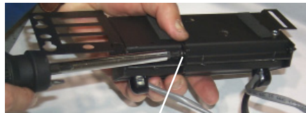
Secure the 2 boxes together with one screw.
