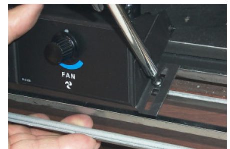
Secure right side with one screw.
