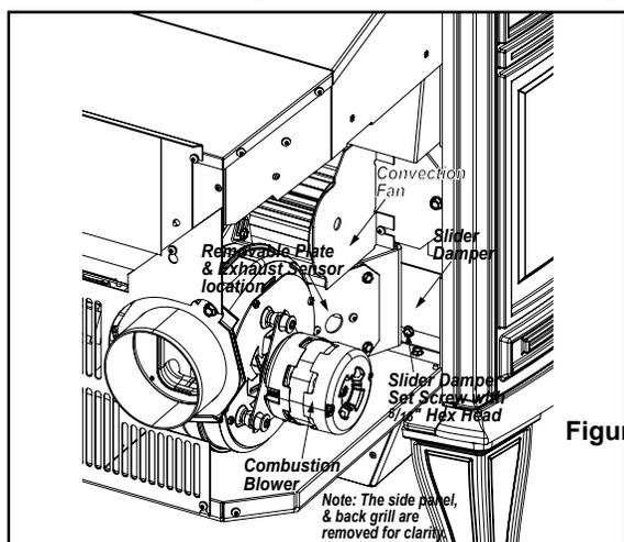
Figure 6: Slider/Damper Plate in Unit.
