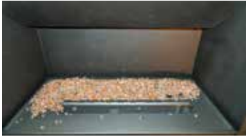
1) Start installing Crystals on back of Burner and Firebox Floor
