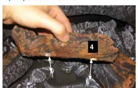
9) Ensure the contour of Log 4 matches up the burner contour and does not rock when seated.
