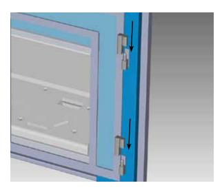
5) Install the supplied bracket in the center of the low lip on the unit base - secure with 2 clips as shown below.
