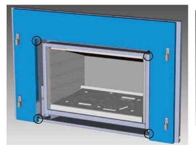
4) Install the optional full screen doors onto the frame.
