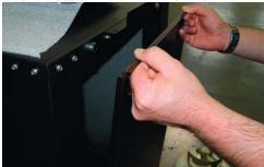
Remove long side panel (left panel if facing ON/OFF switch end), to access the 3/8" fitting to the gas control.
