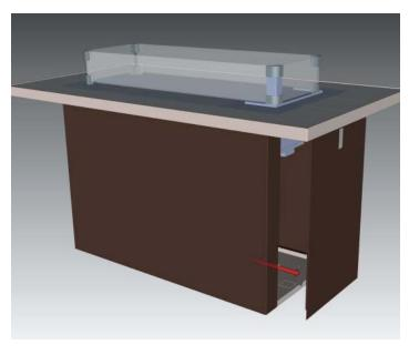
2) Remove two screws to remove valve cover panel in locations shown below.
