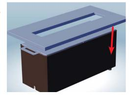
6) Secure table to unit from underside, with 4 screws in locations shown below.
