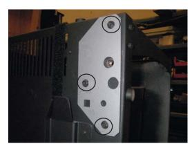
Line up caster with existing nutsert (retrofit) or corresponding hole (see above diagrams) on plate.
