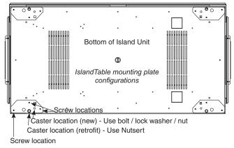
4. Retrofit - Thread bolt into nutsert, hand tighten and finish tightening bolt with supplied allen key.
