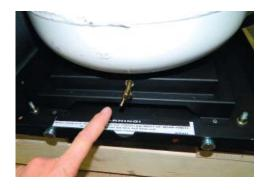
5) Connect the LP regulator quick connect to the tank.
