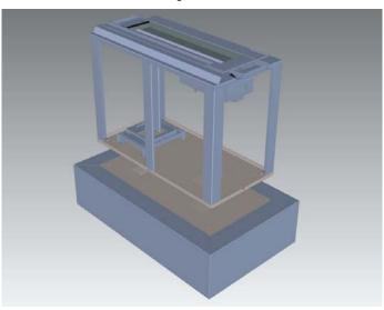
7) If using unit with a natural gas connection, position riser with gas line knockouts over gas supply connection - unless using the LP tank.
