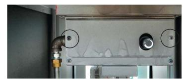
11) Remove Hi/Lo pressure regulator by removing 2 screws as shown below. Reverse steps to install LP pressure regulator. 14) Remove NG gas line, if installed - replace with LP regulator and quick connection.
