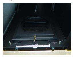
4) Seat tank on tray and tighten butterfly bolt to secure tank to tray.
