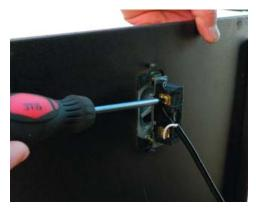
3) Remove 2 screws from switch cover to release switch.
