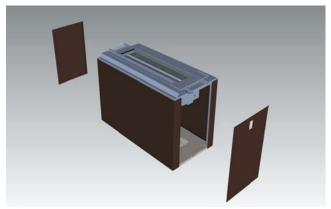
Remove the end panels and long side panels, place on a clean soft surface.
