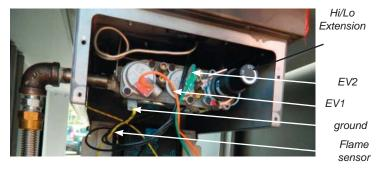
7) Remove 10 screws in locations shown below to remove valve tray.
