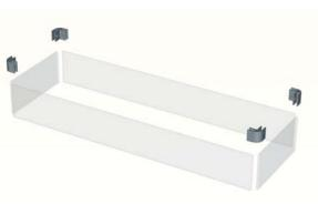
3. Using a flat screwdriver, secure 4 top corner brackets with nylon
