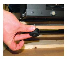
5) Install the 4 adjustable rubber feet into the bottom of the island riser. Seat all the way in and hand tighten.
