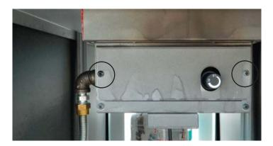
3) Remove two screws to swing down DFC box.
