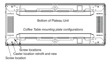
2. Line up mounting plate at each corner on bottom of unit. Secure with three self tapping screws in locations shown below.
