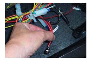
Connect the male end from AC adaptor to the female end tagged "DC Supply" on wiring harness in unit.
