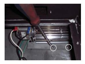
13) Attach the green ground wire to the ground lug - located in the lower left back corner of the unit.
