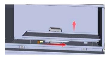
Remove the valve access plate by undoing the 17 outer screws - see locations below.
