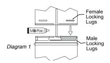
NOTE: For best results and optimum performance with each approved venting system, it is highly recommended to apply "Mill-Pac" sealant (supplied) to every inner pipe connection. Failure to do so may result in drafting or performance issues not covered under warranty.
