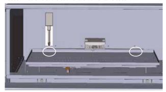
5. Remove the burner by sliding it to the right - then lift out.
