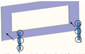
3. Install the glass surround to the unit by hooking the left and right side mounting brackets into the mounting slots at the side of the firebox as shown below. It is recommended that you use the first mounting
