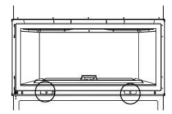
5. Remove the burner tray cover by lifting up and out as shown below.
