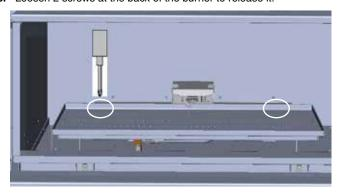
7. Remove the burner by sliding it to the right - then lift out.
