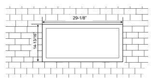
If finishing the unit with the inner faceplate only - the finishing material may be brought up to the edge of the unit.
