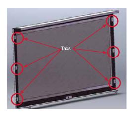
3. Hook the inner door frame (3) and screen assembly (2) over the inner door trim (1).
