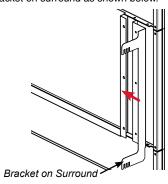
2. Secure with 3 screws for each bracket in locations shown below.
