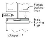
Assemble the desired combination of pipe and elbows to the appliance adaptor and twist-lock for a solid connection.
