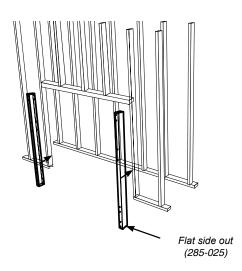
**5**. Secure horizontal steel header stud *(285-026)* with 2 screws per side as per diagram.
