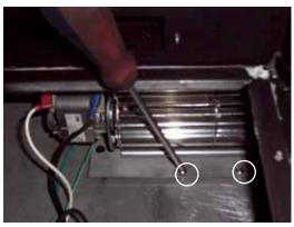
11. Connect the Black wire to the fan motor spade and the other end of the black wire spade to the thermodisc.
