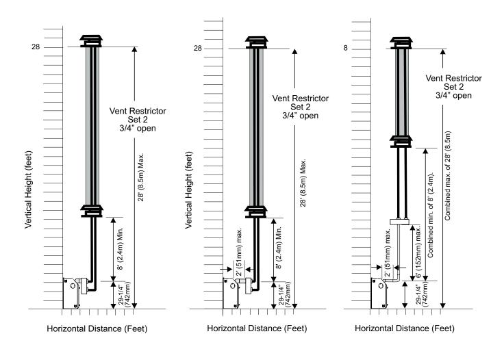
The shaded area in the diagrams shows the allowable vertical terminations when using two 3" co-linear aluminium flex and  $4 \times 6-5/8$ " rigid pipe.
