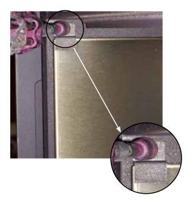
4) Install the right side panel - secure in position with one panel clip and one screw.
