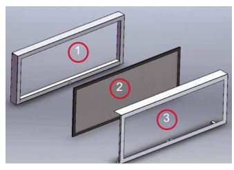
2. Install safety screen (2) into inner door frame (3). Secure screen by bending down the 6 tabs as shown
