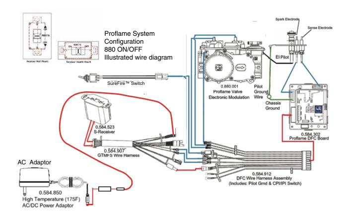
**Note:** Either 4 AA batteries or AC adaptor must be installed to operate the burner switch/Receiver.
