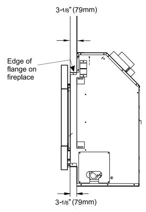
Important: 1/2" gap required between faceplate and finished wall when using part #318-924, 318-927, 316-951, 316-955 (4 pc. faceplate Verona surround). When using part # 316-934 and 316-937 (outer faceplate) the 1/2" gap is not necessary.
