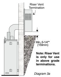
\*Diagrams 3 & 4: As specified in CGA B149 Installation Code. Local codes or regulations may require different clearances.
