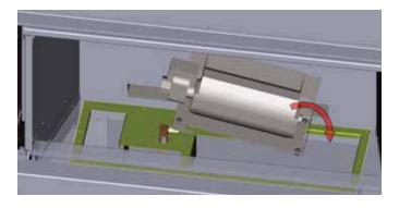
Connect one end of the black wire to the black wire from the power cord.. Connect the other end to one spade on the Fan Motor.
