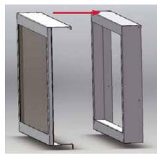
4. Bend the center tab up and secure with a screw to attach the outer frame/safety screen assembly to the inner door trim.
