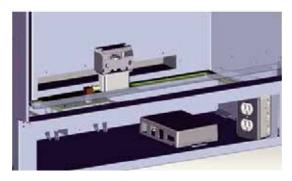
6. Plug in the fan power cord to the Fan Control Module into the outlet marked "Fan". Plug the FCM-COM wire from the remote control wiring harness into the location on the Fan Control Module marked "COM". Turn the switch on the Fan Control Module to the ON position. ON is to the left. The "O" is the off position
