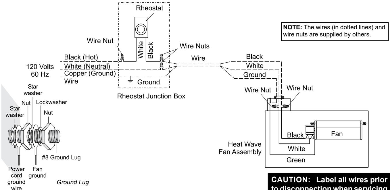
**Caution:** Ensure that the wires do not touch any hot surfaces and are away from sharp edges.
