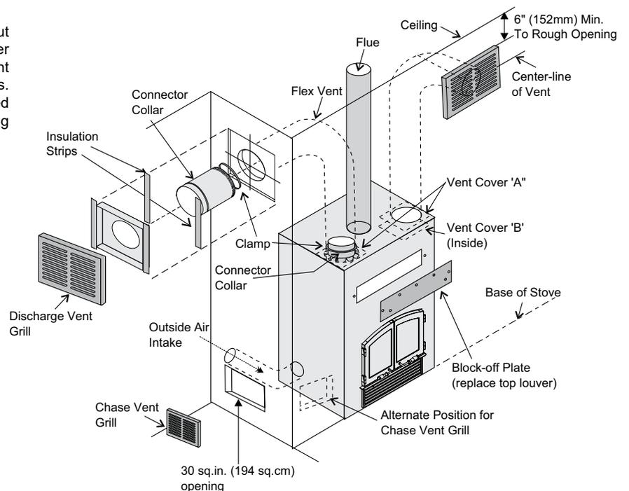
1. Remove the screw from the vent hole cover (vent cover 'A') on top of the unit.
