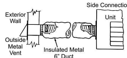
*Outside Air Inlet must be 6 ft. (152mm) below the chimney termination point*
