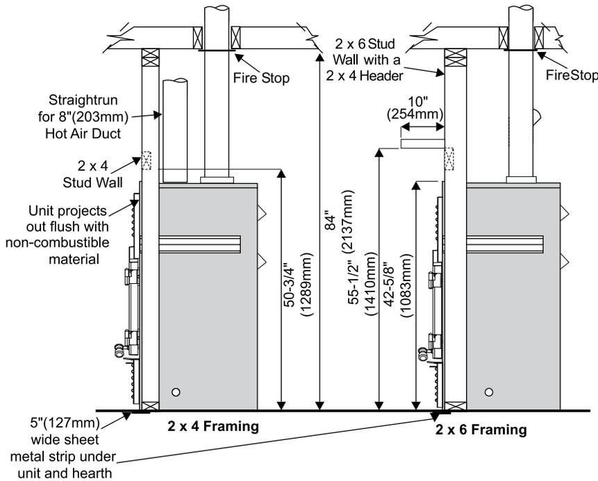
**Note:** The “Z” type safety strip is not supplied by Regency and must be fabricated locally.
