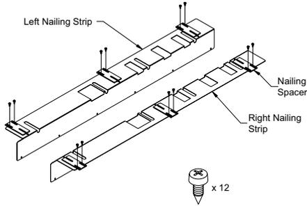
2) Mount Nailing Strips left, right and top to the positions indicated below.
