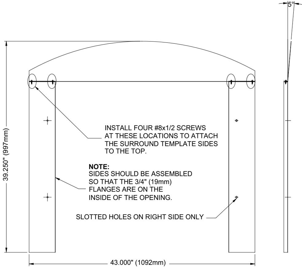
**NOTE:** ONCE THE TEMPLATE IS MOUNTED CHECK TO MAKE SURE THE SIDES ARE PLUMB AND 43" (1092mm) IN WIDTH
