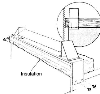
**IMPORTANT: Insulation extends forward to seal against the back of the fireplace masonry or non-combustible face.**
