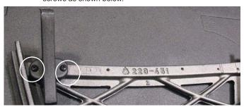
b) Attach bracket to the underside of the side shelf with 2 screws as shown below.
