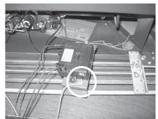
11) Install the supplied battery into the DC Sparker Box by opening the battery compartment.
