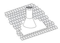
Diagram 10: The upper half of the flashing is installed under the roofing material and not nailed down until the chimney is installed.
