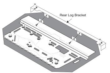
5) Unscrew the 2 Rear Log Pins and move to the front hole position.
