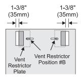
Vertical Termination: Vent Restrictor setting at 36,000 Btu/h
