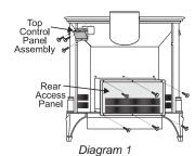
2) Remove the nylon hole plug from the control panel.
