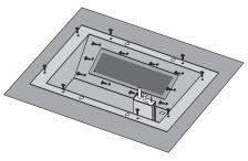
11) Carefully lift the burner tray assembly out.
