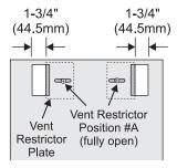
Horizontal Termination: Vent Restrictor setting at 36,000 Btu/h
