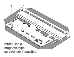
10) Remove all 18 screws holding the burner tray assembly in place.
