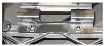
Install 2 screws partially onto bracket in locations shown belowin preparation for installation.
