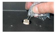
16) Install a gasket over top of the bulb.
