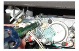
Remove the receiver if installed - unplug the motor wire from the back of the receiver - as shown below.
