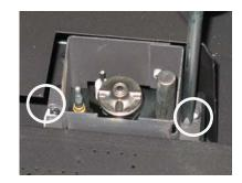
7) Remove the wire clip below the pilot cap.
