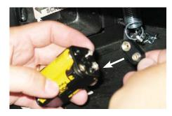
4) Remove DFC (digital firebox control box) from the floor of the unit.
