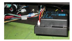
6) Disconnect wire harness, ground wire and spark wire from DFC.
