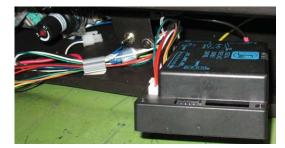
5) Disconnect wire harness, ground wire and spark wire from DFC. See attached wiring diagram for details.
