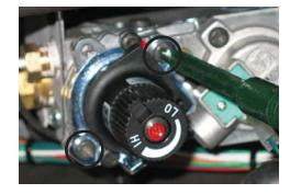
**10)** Install the stepper motor in the same location the hi/lo knob was removed from - with 2 screws as shown below.
