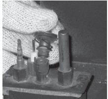
Unscrew the pilot orifice with the allen 9) key; then replace with the LPG pilot orifice, provided in the kit.
