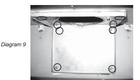
9) From the outside top of the firebox, install the intake collar assembly. Secure with 4 - 1/4" x 1/2" screws. Ensure all screws are tight, but do not over tighten. <u>All 4 screws must be used.</u>
