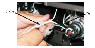
8) Plug in receiver DC supply wire - as shown below.
