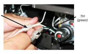
8) Plug in receiver DC supply wire - as shown below.
