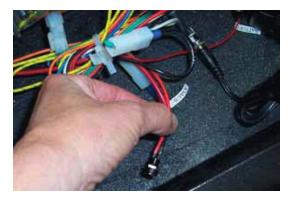
2) Connect the male end from AC adaptor to the female end tagged "DC Supply" on wiring harness in unit.
