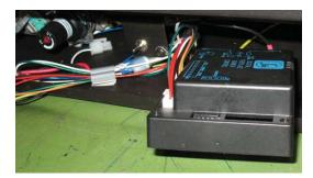
5) Disconnect wire harness, ground wire and spark wire from DFC.
