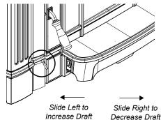
As well as a primary and glass wash air system, the unit has a full secondary draft system that allows air to the induction ports at the top of the firebox, just below the flue baffle.
