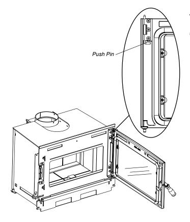
2) NOTE: For Masonry installation make sure that the firebox is level with the hearth using non-combustible materials and no more than 1/2 to 1 inch of the leveling bolt. 3) Lift the unit up onto the Hearth and slide into the fireplace opening. Be sure to leave the unit out at least 3 to 4 inches in order to make the necessary flue connections and to install the fan and faceplate.
