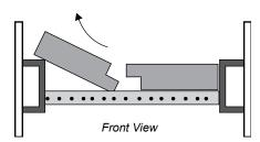
Important: push both baffle bricks so they are tight against the side walls and to the back.
