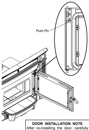
After re-installing the door, carefully swing open and check the clearance to the Right Hand Cast Side. If tight or rubbing, loosen the 7/16 nuts and adjust the clearance and then re-tighten.
