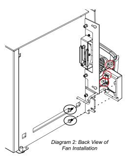
**Note:** If screws do not lineup, loosen the 2 screws per side as shown in Diagram 2 and adjust left side and right side facia. Tighten the 2 screws per side and install the fan on the unit.
