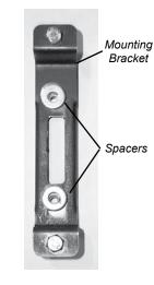
4) Re-secure Latch to Mounting Bracket using 2 bolts
