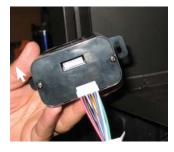
**12)** Connect GTM motor wire from the stepper motor to the wire connector from the receiver wire harness.
