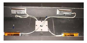
23) Attach ground wire to ground lug - and plug in light assembly.
