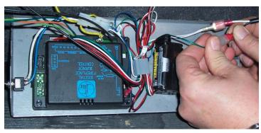
6) Reinstall the module and battery pack tray into the holder
