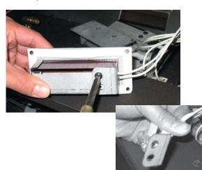
13) Remove the amber glass - by sliding out.
