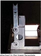
10) With brackets and inner slides attached to the lower faceplate panel - guide the lower faceplate panel into the outer slides located in the bottom part of the unit. See inset. Push in until flush with upper faceplate.
