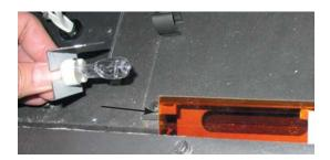
20) Secure socket to light diffuser with one screw - as shown below.
