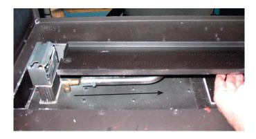
8) Disconnect the ON/OFF connector wires from the valve.
