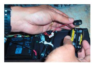
**4)** Install - 4 AA batteries, reconnect the connector to the battery pack and put back onto Velcro strip
