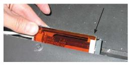
18) Install bulb into socket end of assembly.
