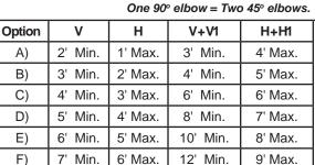
length is 30 feet with minimum of 12 feet total vertical and maximum 9 feet total horizontal.
