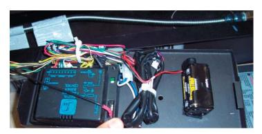
3) Disconnect connector from battery holder and remove from tray – (battery holder is attached by Velcro to tray).
