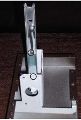
**HZ42ST** - install slider on this side of the bracket.
