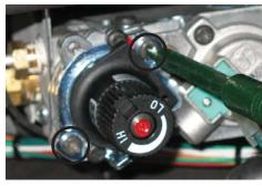
8) Install the stepper motor in the same location the hi/lo knob was removed from - with 2 screws as shown below.
