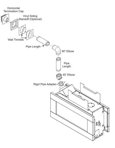
When using Rigid Vent other than Simpson Dura-Vent, 3 screws must be used to secure rigid pipe to adaptor.
