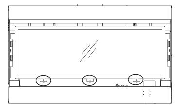
5) Remove bottom cover by lifting up and out.
