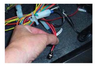
Connect the male end from AC adaptor to the female end tagged "DC Supply" on wiring harness in unit.
