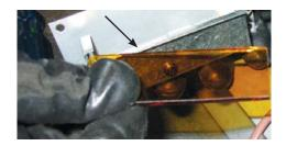
14) Place gasket over the inside perimeter of the light diffuser box.
