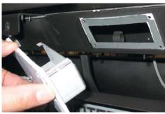
**16)** Secure the light diffuser in place with the 4 screws set aside from the cover plates.
