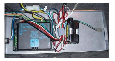
5) Locate the Green and White from the DFBC module wire harness; connect the spade connectors from the On/Off switch. Green to Black and White to White.
