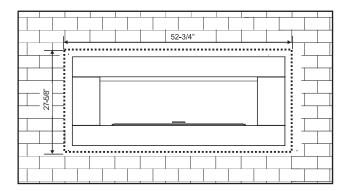
5) For material such as brick, stone, etc that extends less than 1-1/2", the minimum opening dimensions noted below must be adhered, when finishing around the faceplate. This is to ensure the removal of the faceplate and for the safe operation of this appliance.
