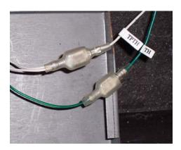
**6)** Locate the DFC wire from the receiver wire harness and connect to the DC supply wire from the DFBC.
