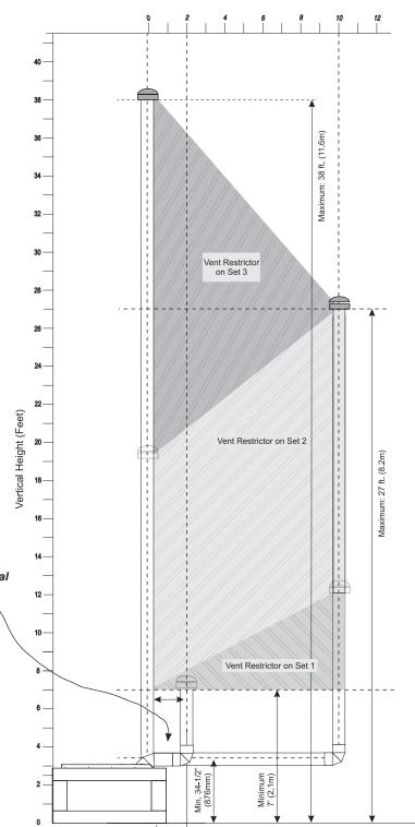
Minimum length of pipe between elbows 12" (305mm)
