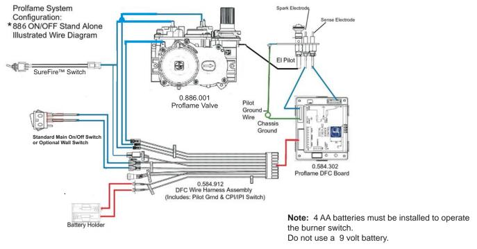
**IMPORTANT:** If the optional remote control is used, the AA batteries normally installed into the battery holder must be removed. The AA batteries in the receiver now operate the unit. Having AA batteries in both the battery holder and receiver will damage the gas valve.
