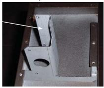
HZ42 - Install slider with flat side facing outward -secure with 2 screws in locations shown.
