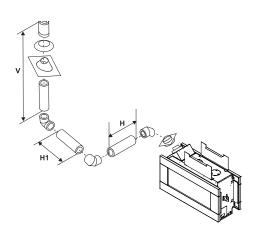
For additional vertical venting with 2 x 90° elbows, refer to "Rigid Pipe Venting Arrangements" Section.
