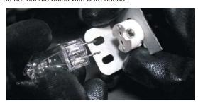
19) Install socket and bulb into light diffuser as shown below.
