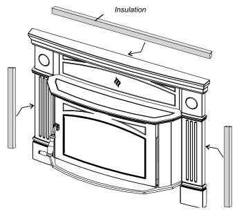
11) The unit may now carefully be slid into final position. See side cast adjustments if faceplate needs aligning.
