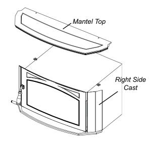
With the Mantel Top in place check to make sure there is no gap between the nut retainer and the underside cast of the Mantel Top. If there is a gap present you will need to lower that side cast by loosening 2 bolts, see step 6 for bolt location (check to see if level).
