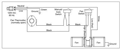
Blower/Fan Wiring Diagram
