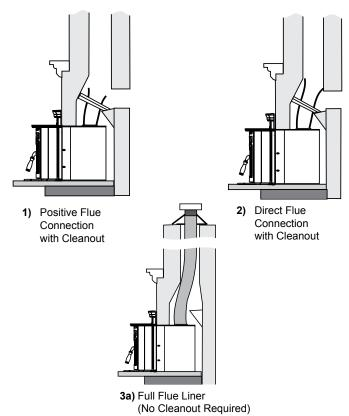
Note: A clean-out door is sometimes required, by your inspector, to be installed when either the Positive flue connection or Direct flue connection method is used.
