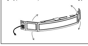
3) Ensure the power cord and all other wires will not come into contact with any hot stove surfaces.
