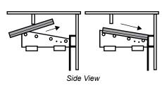
Tilt the left baffle up on top of the side channel and it will leave enough room to position
