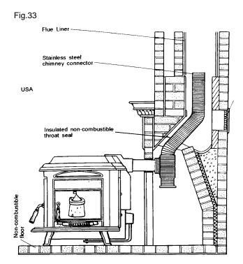
In Canada when connecting to a masonry fireplace the steel chimney connector must terminate at the top of the masonry chimney or flue liner.
