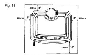
If the side door is to be used the floor protector must extend at least 18" (450mm) from the right side of the stove when looking from the front.
