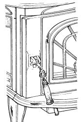
h) If the side fuelling door (item 21) is to be used, fit the side ash lip (item 24) using two ashlip brackets (item 35) and screw together using four 1/4" (6mm) x 1/2" (12mm) hex head bolts provided. Take out the chrome locking bolt and fit door latch (item 73), the door latch spigot (item 40), and the wooden handle (item 28) provided.
