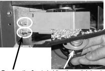
Remove the 2 nuts holding the switch box in place, then pull the thermosdisc out of the bracket.
