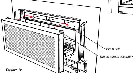
**12.** Lower screen assembly onto unit, bottom of screen is secured by 2 magnets
