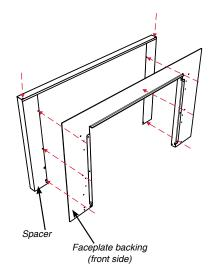
2. Install the custom backing plate to the faceplate backing and spacer with 9 screws (3 on each side and 3 across the top) installed from the backside of the backing plate into the backside of the assembled faceplate backing with spacer as shown below.
