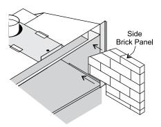
Note: Use caution when sliding side panels in as they can easily be scratched by the brick panel tabs.
