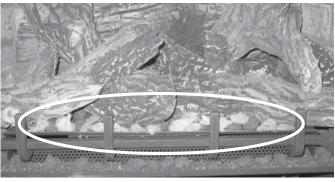
13) Separate platinum embers and place on the burner just in front of the logs. Avoid stacking platinum embers.
