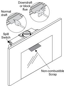
a scrap piece of sheet metal (or other noncombustible material) in the space between the glass door and faceplate, this will prevent the natural convection of the unit from interfering with the test.
