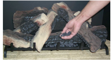
Place embers on the burner tray. DO NOT BLOCK BURNER HOLES
